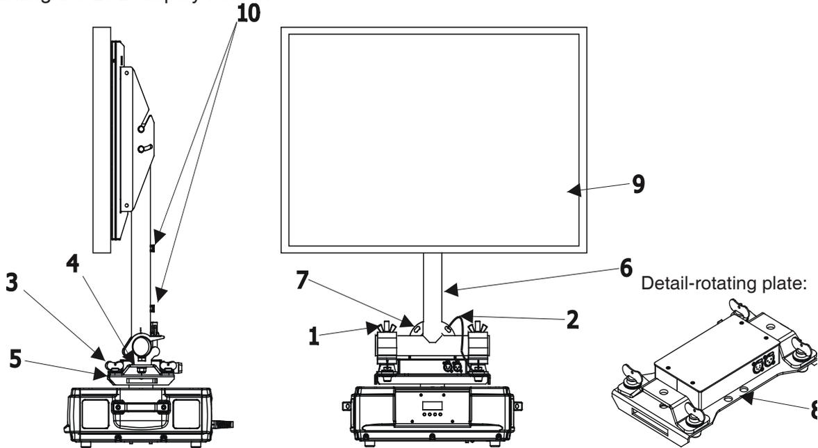
1. Bolt two clamps (1) to the omega holders (4) with M12 bolts and lock nuts through the hole in the holders.
