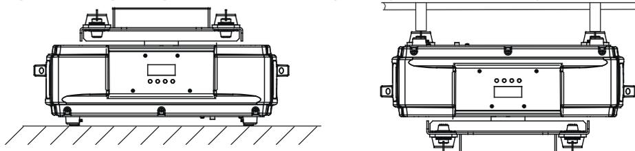
For overhead use, always install a safety-rope that can hold at least 10 times the weight of the device. You must only use safety-ropes with screw-on carabines. Pull the safety-rope through the two apertures on the bottom of the base and over the trussing system etc. Insert the end in the carabine and tighten the fixation screw.
