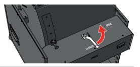
4 Move the manual CO<sub>2</sub> valve back in CLOSED position.
