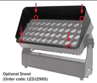
To fit the snoot, place it over the front lens of the fixture and use the four thumbscrews located in each corner to tightnen it to the fixture.
